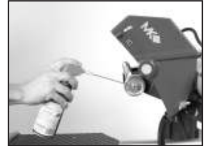
(C) Lubricate the Arbor Shaft.
