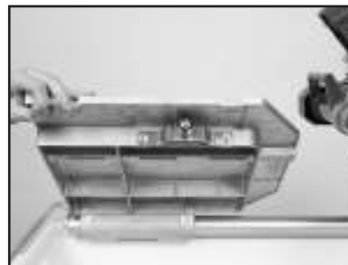
(B) Check the Movable Cutting Table Roller Wheels for wear – replace if necessary.
