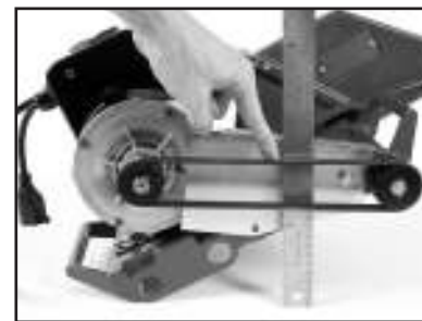
(F) Check belt for proper tension. If tension correct, go to step Q (proper tension should be 1/8-inch deflection)
