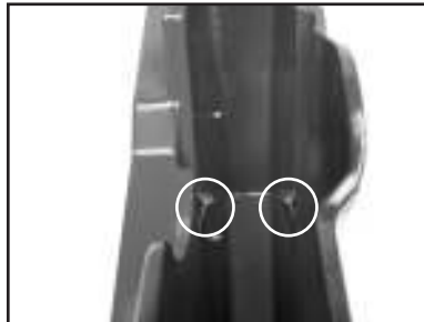
(B) Run the saw until clear water is seen at the blade cooling ports (Approx. 1 minute).
