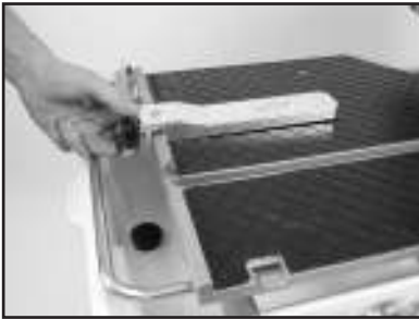
(A) Remove the Adjustable Cutting Guide.
