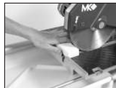
(C) Position the Dressing Stick. Cut 2 or 3 strips from the dressing stick to dress the Blade.
