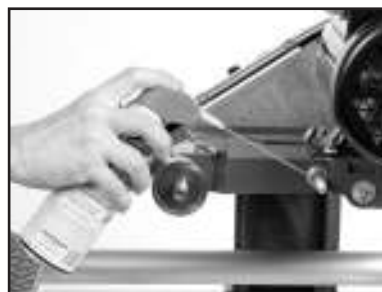
(H) Lubricate the Blade Guard Pivot Shaft.
