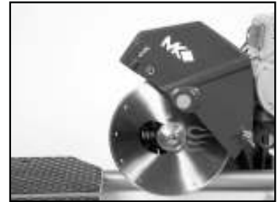
(C) Inspect the Diamond Blade for damage – verify the blade is correct for the material being cut.
