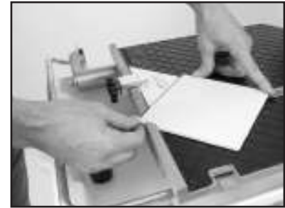
(C) Position the tile against the Guide and Ruler/Stop. Turn the motor on.
