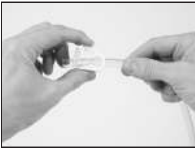
(A) Verify the cooling flow Adjusting Clamp is open. If flow exists, go to Step B.
