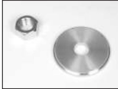
(B) Lubricate the Outer Flange and Retaining-nut.
