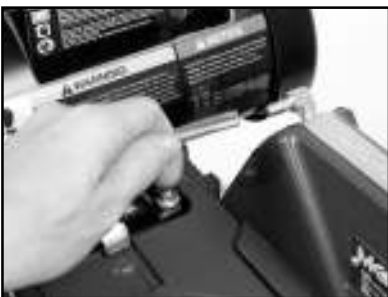
(A) Connect the Cooling Transfer Tube to the inlet connection of the Blade Guard.
