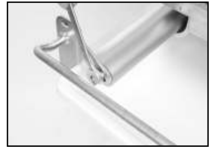
(C) Loosen front and rear Guide Bar Retaining Bolts.
