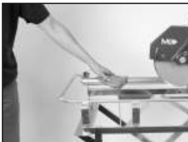
(A) Check the Guide Bar and Frame for cleanliness – clean if dirty.
