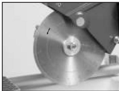
(B) Check for proper blade rotation.
