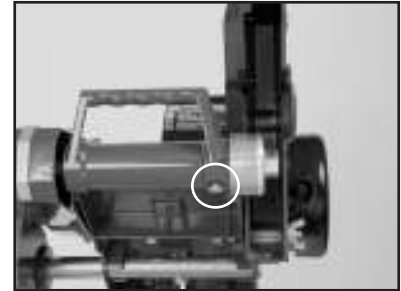
(C) Locate the Shaft Lock push button on the underside of the Cutting Head.
